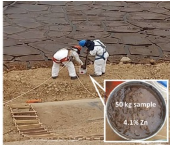
Figure 1. Historical Gypsum Tailings Pond at Nexa, Cajamarquilla (Top) and sampling of the top one meter done by Nexa in March 2022 (bottom).
